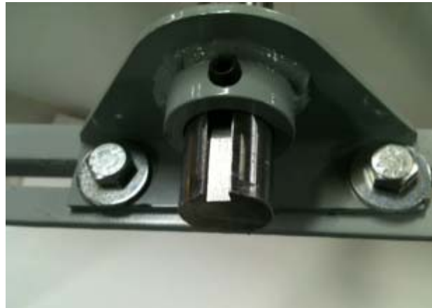
Shaft Retainer Bracket used with Balancing Spring
