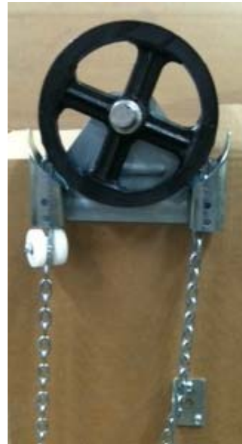
Chain hoist showing Chain Stop and Stop block installed
