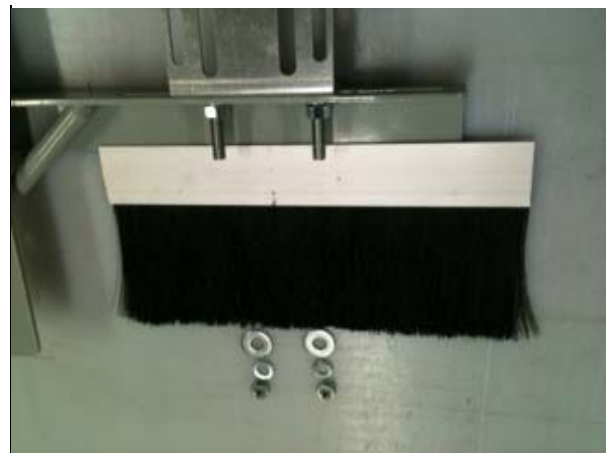
Top side brush seal and fasteners
