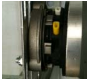
Limit switch adjustment buttons. Cover shown removed.
