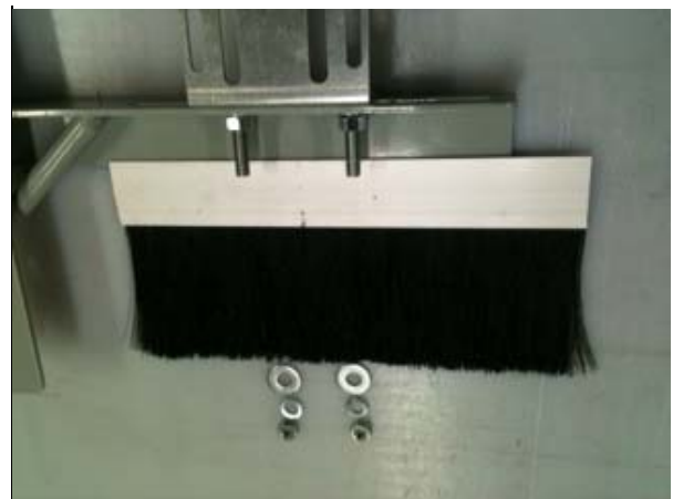
Top side brush seal and fasteners
