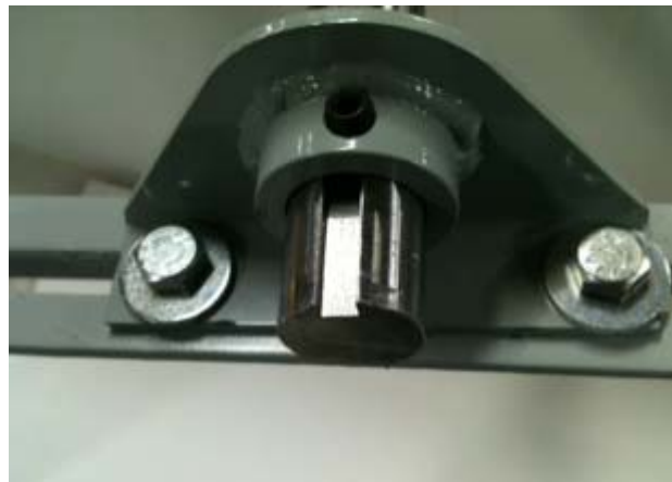
Shaft Retainer Bracket used with Balancing Spring
